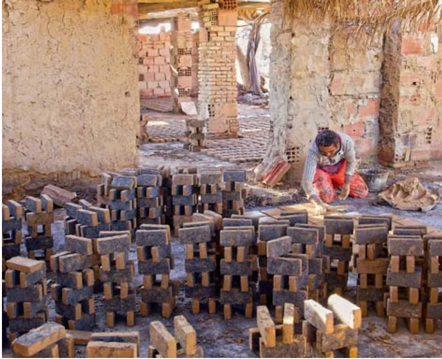
Surrounded by stacks of drying bricks, eighth-generation Tozeur brickmaker Antar Chorba pushes a wet mix of clay into block form as many as 600 times in a day. The bricks dry in stacks that will later be fired.
